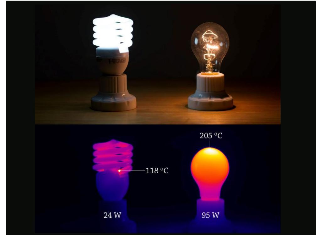
Thermography image of CFL lamp vs incandescent lamp
