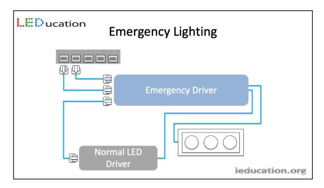
One example on the market today, where two runs of cable from the switch are used. One is to provide pass through power to a normal PoE LED driver, and provide that monitoring of power, while the second run from the PSE provides the charging circuit for an onboard battery. The device then provides the UL924 bypass like a typical unit device, moving the LED array onto the battery
