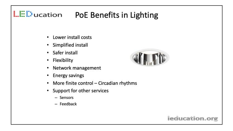
Lower install costs. Cat5e or Cat6 cable is being used to transmit the signal and power, with that cost compared against the use of THHN conductors and a separate control cable for the luminaire control. There is a lot of discussion with regards to the labor side of the installation, with an electrician on the line voltage install vs a data technician for the category cable installation, but one thing to keep in mind is you don't completely remove the electrician from the equation.
