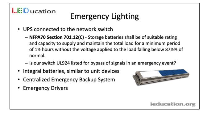
Your usual UPS is not designed around this requirement, it is designed to sustain for a shorter period of time and allow for an orderly shut down of a system.
