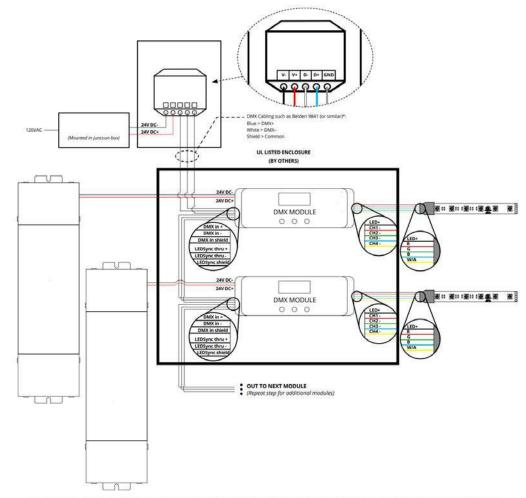
ALL DMX CABLING SHALL CONFORM TO ANSI E1.27-2-2009 (R2014), RECOMMENDED PRACTICE FOR PERMANENTLY INSTALLED CONTROL CABLES FOR USE WITH ANSI E1.11 (DMX512-A) AND USITT DMX512/1990 PRODUCTS.
