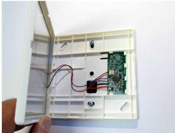
3. Align Bezel to mounting frame, snap in place
