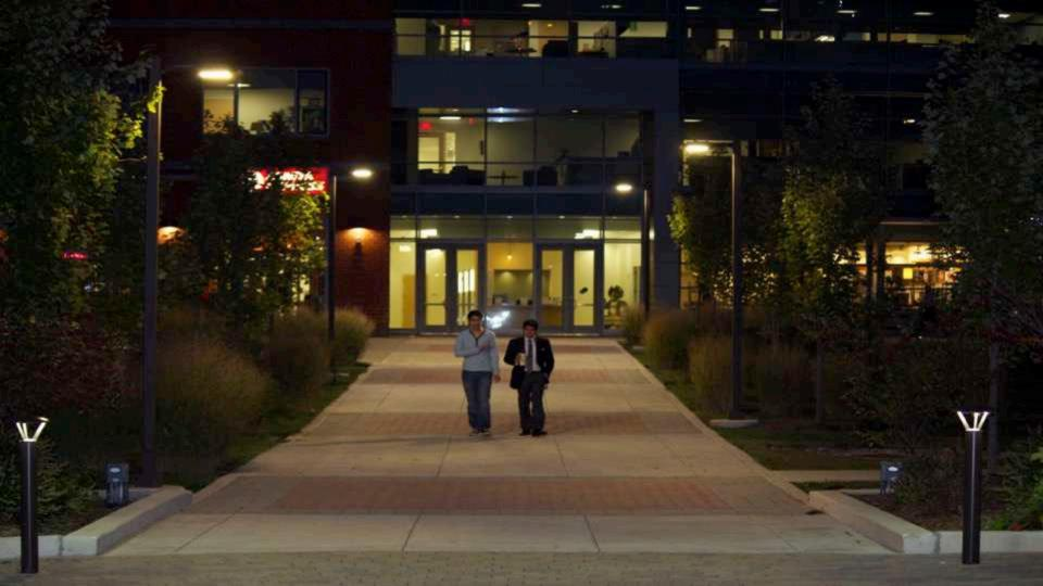
**Visual Comfort** Using appropriate BUG rated fixture reduces adverse impact and improves visual comfort Uniformity doesn't trump glare/light trespass Point source LED without diffusion reduces visual comfort, especially for pedestrians Plenty of fixtures with improved visual comfort available now
