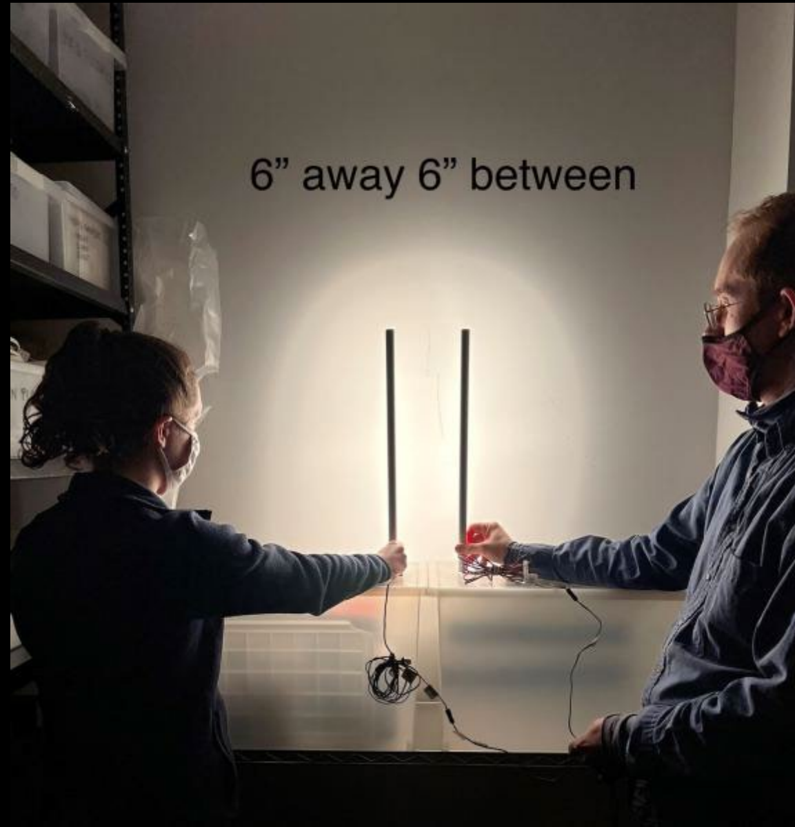
IN-HOUSE MOCKUP TO TEST LUMINAIRE AT 6" FROM WALL AND 6" BETWEEN.
