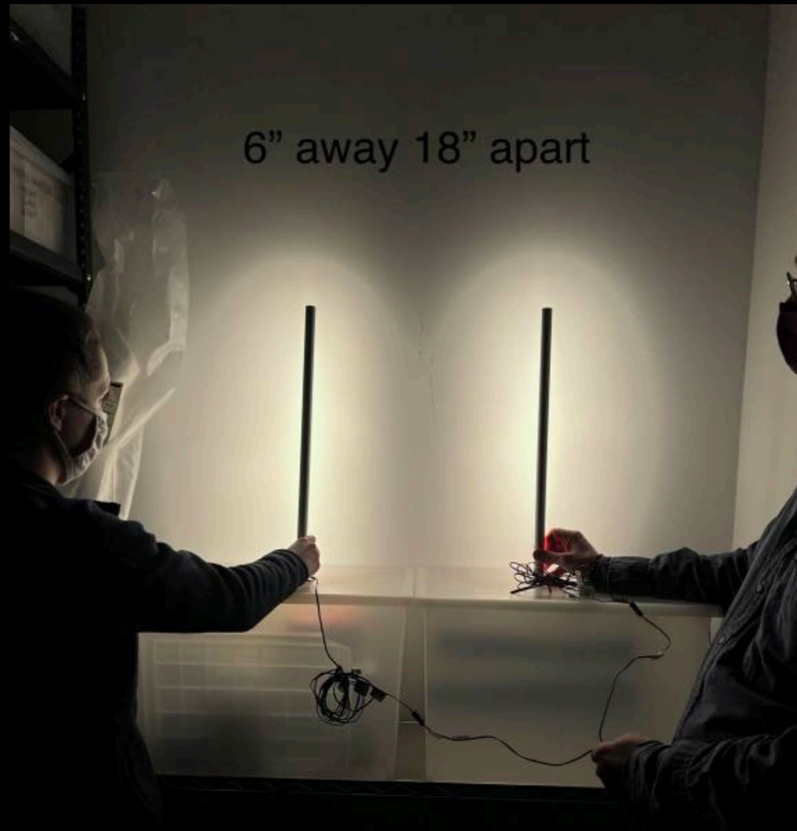
IN-HOUSE MOCKUP: LINEAR LED LIGHTS WALL AT 6" AWAY FROM WALL AND 18" APART.
