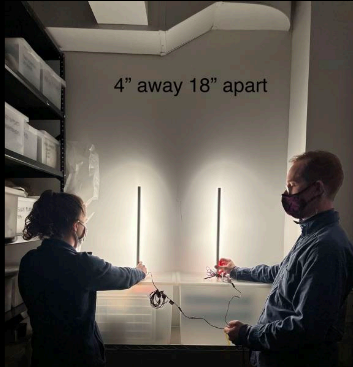
IN-HOUSE MOCKUP TO TEST VARIOUS ORIENTATIONS OF THE SELECTED LUMINAIRE.
