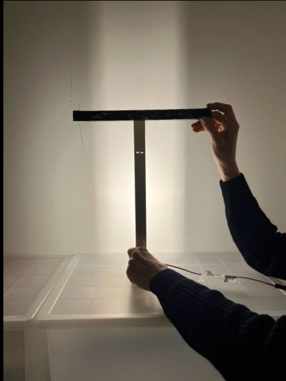
IN-HOUSE MOCKUP TO TEST VARIOUS ORIENTATIONS OF THE SELECTED LUMINAIRE.
